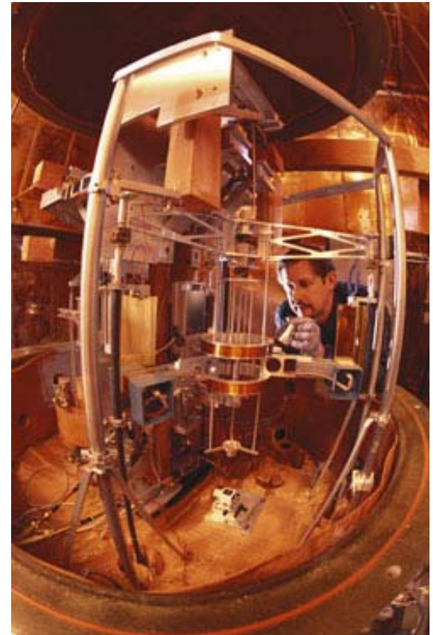
Physicist Richard Steiner adjusts the electronic kilogram, an experimental apparatus for defining mass in terms of the basic properties of nature.
