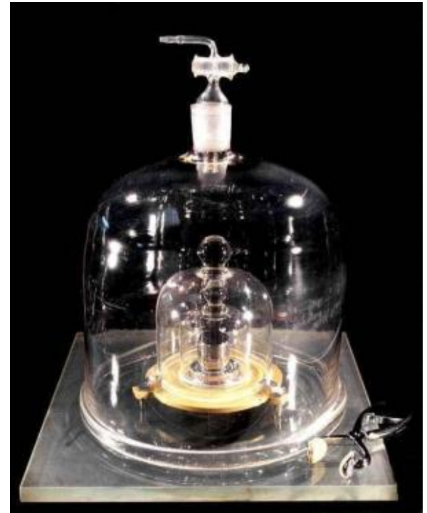
The international prototype of the kilogram in Sèvres. (Credit: Image courtesy of BIPM)
